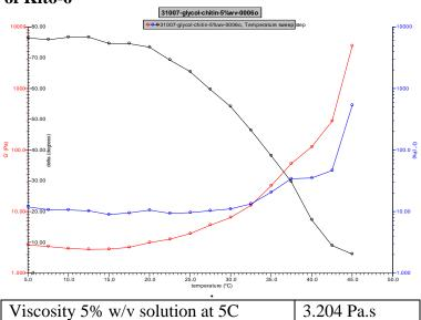
Rheology performed on AR550 (TA instruments) with 60mm 2° cone on 5% w/v polymer in water dissolved at a minimum of 24hrs with stirring at 4C. Viscosity of solution at 0.1 (sec-1) and 5C was measured (1minute peak hold 5 second test intervals). Rheology performed by oscillating at constant 6.283 rad/s, 0.1% strain, in increments of 2.5C ranging from 5-45C with 3 minutes of temperature equilibration at each point.
